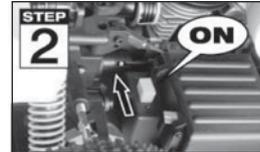
After the transmitter is on, turn on the receiver.
