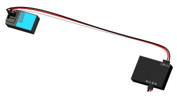
Your third channel needs to be a three position switch in order to fully operate the winch properly.
