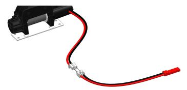
2. Plug winch/control box plug into control box marked W+/W-. (Check Direction of your wires and plug, Red +, Black -)
