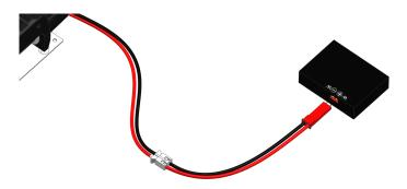
Connect the receiver wire to the control box marked B+/B-. (Check Direction of your wires and plug, Red +, Black -)
