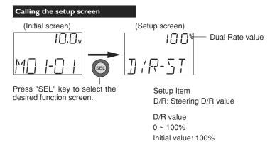
When Dual Rate lever is operated, the "D/R-ST" screen is displayed automaticaly for about three seconds.
