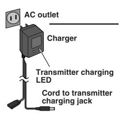
When charging the NT8F700B NiCd battery with the special charger, allow about 15 hours for charging. If the transmitter has not been used for some time, cycle the battery by charging and discharging it two or three times.
