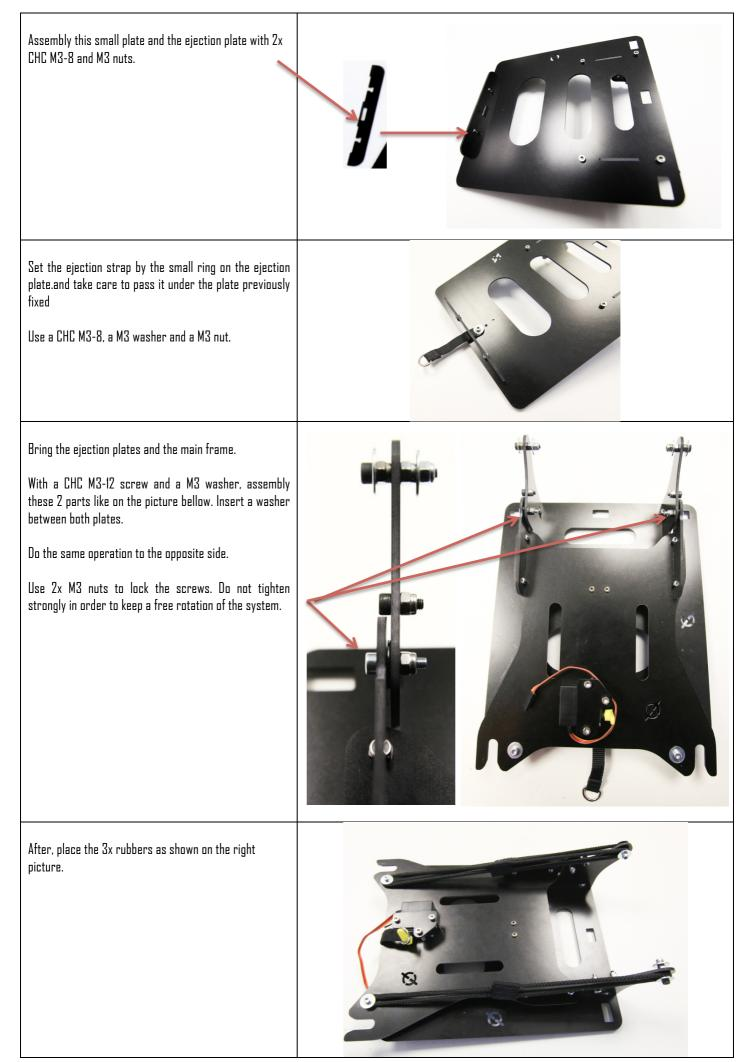
One time the rubber is installed, bring the Pod L2 and set it on the ejection plate.
