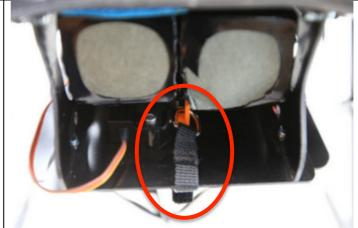
Mount the long straps on the motor arms basis. (one on the left, one on the right)
