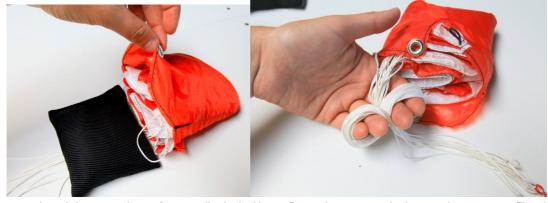
Grab the lines and wind them round your fingers till it looks like an 8 in order to store the lines in the container. Then house the lines inside the container just in front of the parachute's trailing edge.
