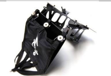
Remove the landing gear from the multirotor main frame. Depends on the use (with or without gimbal), place the rescue system correctly in order to have the right center of gravity (the landing gear has to stay perfectly horizontal) Here on the picture, there is any gimbal, then we place the rescue system on the center. If we put a gimbal on the front, the rescue system will be on the back.
