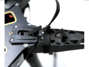
After, place the main rescue strap in the 2 straps loop which are on the multirotor frame. Now the assembly of straps looks like a Y.
