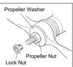
Obviously, this can be very hazardous. To eliminate such dangers, the O.S. Safety Locknut Assembly was devised. Install this as follows:
