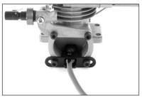
**Note:** On some engines you may need to space the sensor further away from the backplate. The sensor picks up the crankpin only; on some engines if the sensor is too close, it will not distinguish the crankpin from the crank weight.
