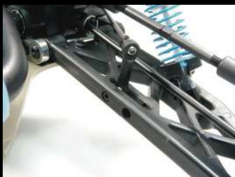
Front and Rear Arm Adjustable Sway Bar System
