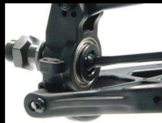
Oversized Bearings in Front and Rear Hub System
