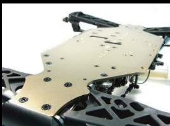
Professional 3mm Aluminium Hard-coated Chassis
