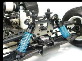
3mm T6 7075 Front and Rear Shock Towers
