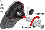
high-pitch, whining noise. Remove the rubber slipper clutch plug on the transmission cover in order to adjust the slipper. Use the 4-way wrench to turn the adjusting nut clockwise to tighten and counter-clockwise to loosen. Place the model on a high-traction surface, such as carpet. Adjust the slipper so that you can hear it slip for approximately two feet from a standing, full throttle start. (Learn more about adjusting the slipper clutch in the sidebar.)
