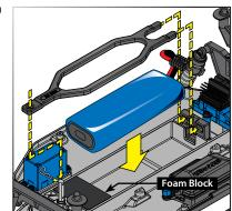
post. Secure the battery hold-down with body clip in the hole in the post. Do not connect the battery pack yet.
