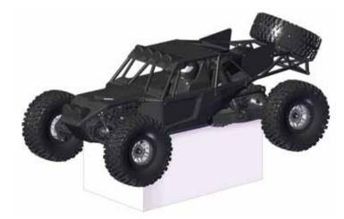
Perform a control test with the vehicle wheels off the ground. If the wheels rotate after the vehicle is powered ON, adjust the "TH. Trim" knob until they stop. To make the wheels move forward, pull the trigger. To reverse them, wait for the wheels to stop, then push the trigger. When moving forward, the wheels should maintain a straight line without any steering wheel input. If not, adjust the "ST. Trim" knob so the wheels maintain a straight line without having to turn the steering wheel.
