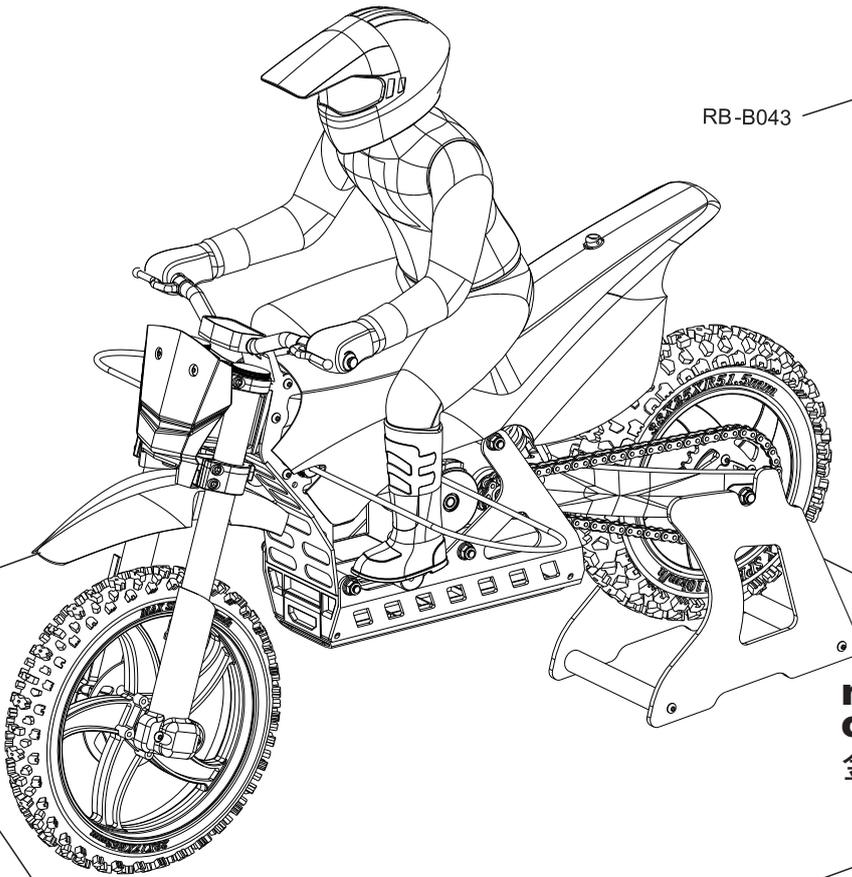
**Caution:** Before you power on the bike, please make sure the bike stand of the bike is not on metal or conductive surface, unless it may cause short circuit and the ESC may get burnt when the gyro starts
