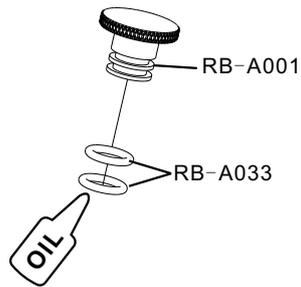
**Note:** It will be easier to assemble if you add oil to the ring (RB-A033) before installation.
