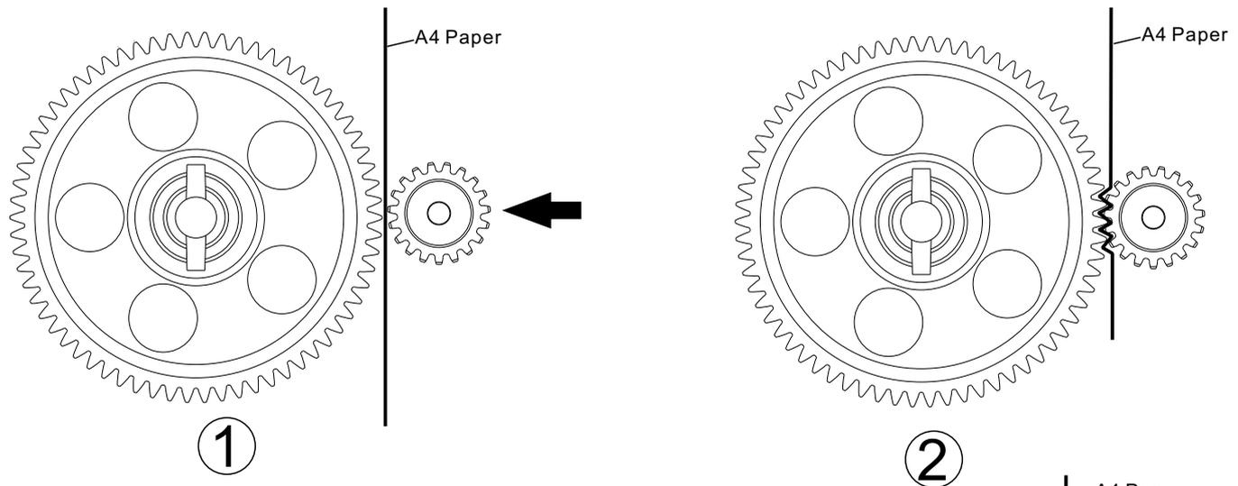
**Caution:** The space between the two gears should be the same thickness as one piece of A4 paper. We can put one piece of A4 paper between the two gears before assembly and take it away after finish.
