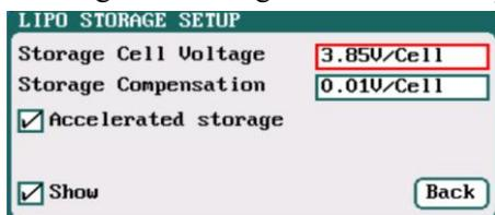
Storage Cell Voltage: 3.7V/Cell-3.9V/Cell;
