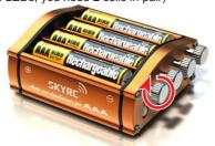
3. When LEDs turn off, please unscrew 4 screws and take out the batteries from the tray.
