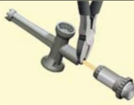
C. Remove/Install Rod End
