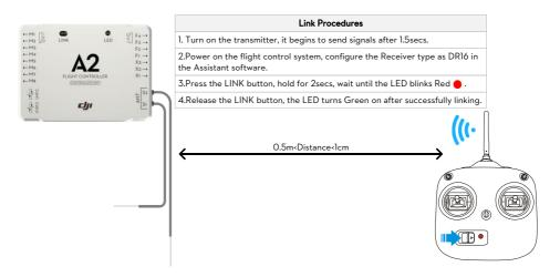
The DR16 Receiver is compatible with the Futaba transmitters which have optional FASST MODE MULT, MLT2 or 7CH. Users can find out the available Futaba transmitters and configuration requirments a dhere to the FAQ->The Transmitter setup of FUTABA.
