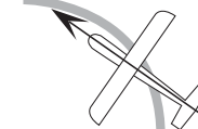
Nose Points inside circle Too much coupling or differential. Reduce one or both.
