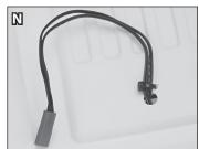
5. Next, route an included zip tie through one of the small holes from the inside of the body. Fold the zip tie over and through the other small hole on the top of the body (M). Secure the light wire to the inside of the body by tightening the zip tie (see N for correct orientation). Make sure to leave some slack
