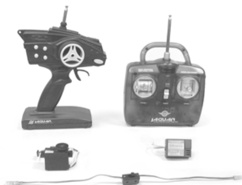
2-Channel Surface or Pistol Radio with Standard Servo. 2動作發射機、接收機及伺服機
