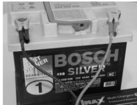
Using terminal clip attaching to car battery
