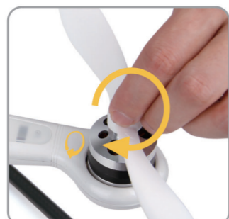
1.2 Follow the principle of propellers' arrows consistent with body arrow marks to assemble clockwise and counterclockwise propellers.
