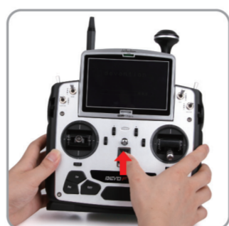
2.3 Turn all the Switch of transmitter to "0" Position, push the throttle stick to the lowest position, Turn on the transmitter power.
