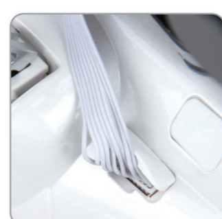
4.5 Insert 9 pin of the Gimbal date wire into the Gimbal connection port at the bottom of the aircraft.
