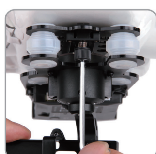
4.4 Put the spring into M3x12 screw, aim to the threaded hole, tighten up the screw to Gimbal.
