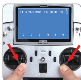
3.1 Enter into Compass Calibration, Aircraft red, green LED light flash quickly.
