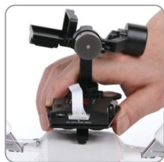
4.3 Put the Gimbal sliding chute aim to gimbal fixed block, and enclose to the bottom of gimbal fixed block.
