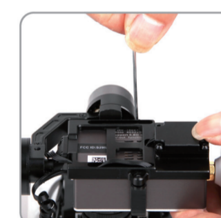
5.3 Install the camera into gimbal, Fix it with camera fixed frame (ensure the gap close to the lens), then screw the M2x4 screw to the camera fixed frame again.
