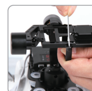
5.2 Unscrew 2 M2x4 screw, Loosen the camera fixed frame.
