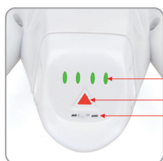
2.4 Turn the power switch to "ON" position, and press on the power button about 3-5 second till the green LED light solid. The undercarriage(skid landing) will unfold automatically.
