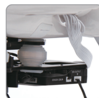
5.4 Insert the camera power cable into power output port of G-3D.
