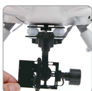
4.6 G-3D Gimbal Installation finished.
