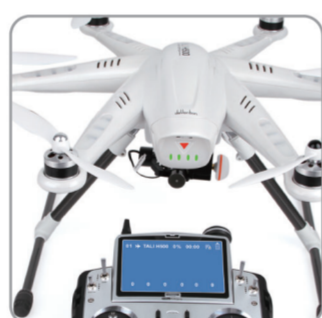
3.6 Put aircraft to the horizontal position, the Red LED and Green LED light out which means calibration finished. Please reconnect the aircraft power after calibration.
