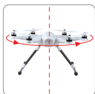
3.4 Horizon level 360° rotation (Rotate the aircraft, from 0° to 90°, 180°, 270°, 360°, all need to pause for 1 second.)
